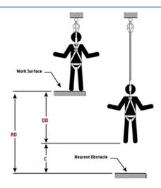
DD = Free fall, lock off and deceleration (1.4m) + Dring slide and harness stretch (0.25m)
